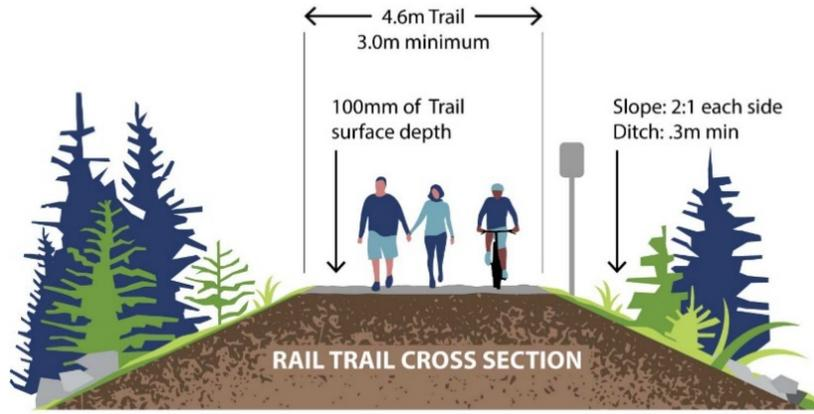
Reshape and compact existing subgrade to allow for drainage to be directed away from all bodies of water
